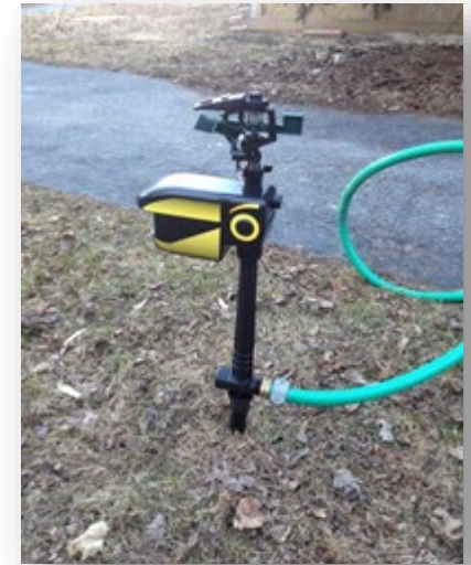
The Scarecrow® motion-activated sprayer connects to your garden hose and frightens approaching geese with a sudden blast of water
